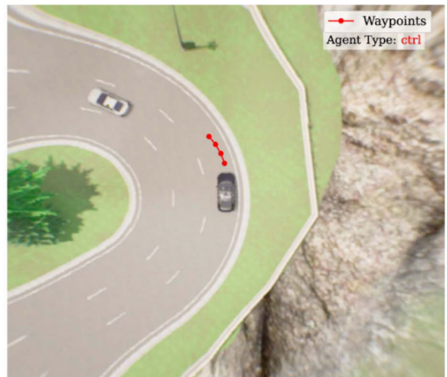
FIGURE 8. An example image from Azam and Kyrki [117] demonstrates how waypoint representations are interpretable and can be viewed in BEV space.
